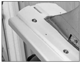
Carefully place the main plate in position under the L/U cav plate and then put on the upper plate, aligning the holes, sandwiching the L/U's cav plate between them.
