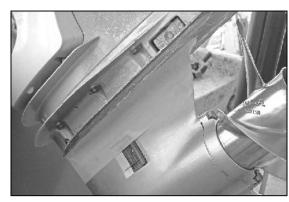
The larger plate is the "main" plate and the smaller is the "upper" plate.
