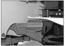
The ideal position for the cav plate with the motor in its correct position can be determined by using a long straight edge, yard stick or similar straight object and placing it inside the top of the tunnel extending out under the cav plate to determine where the water flow will hit/contact the underside of the cav plate. The best place for the water to contact the cav plate is several inches behind the nose of the cav plate with the motor trimmed level.
