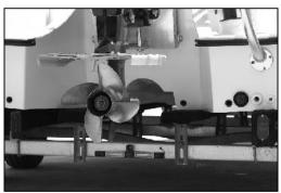
You may need to adjust the height of your motor (normally higher than where it was mounted before installing a cav plate) in order for the tunnel water stream to contact the cav plate underside at the proper spot.
