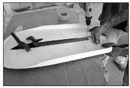
Double check alignment, and using a 1/4" drill bit drill one of the back corner holes, and pin it in place using one of the supplied bolts. Continue drilling the corner holes one at a time, pinning them as you go to make sure the plates don't change position. Once all of the 4 corner holes are drilled, just drill all of the remaining holes.
