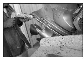
Also, place a bead of silicone on the top of the motor's lower unit metal cav plate out by its edge.
