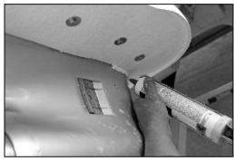
Using silicone, you will need to seal the openings at the nose and rear of the cav plate.
