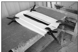
Assuming that your alignment marks and back edges of the plates are correct, remove the plates and place them together in their proper positions. Using large spring clamps, clamp the plates together, two on the front and two in the back. What you're doing is using the main plate as a pattern for drilling the upper plate holes so alignment and positioning is critical.
