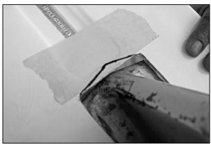
The metal cav plate on most outboard lower units is basically square across the back. However, in some cases it may be rounded or pointed. So, to prevent water from splashing up from this area, the back of the upper plate's center cut-out must be shaped as closely as possible to that of the L/U cav plate back end.
