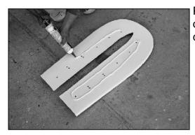
Put a thick (1/4" to 3/8") bead of silicone on the top of the main plate next to the center cut-out and close to the outside of the holes as shown.
