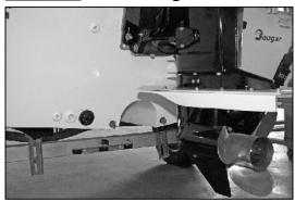
For best performance, the cavitation plate should be approximately 3/4" or higher above the "water stream" exiting the boat's tunnel. If your boat is not equipped with a jack plate, that height will normally be about 3/4" to 1" above the tunnel. Boats equipped with a jack plate will require that the cav plate be higher, typically about 2" for every 5" of jack plate setback.
